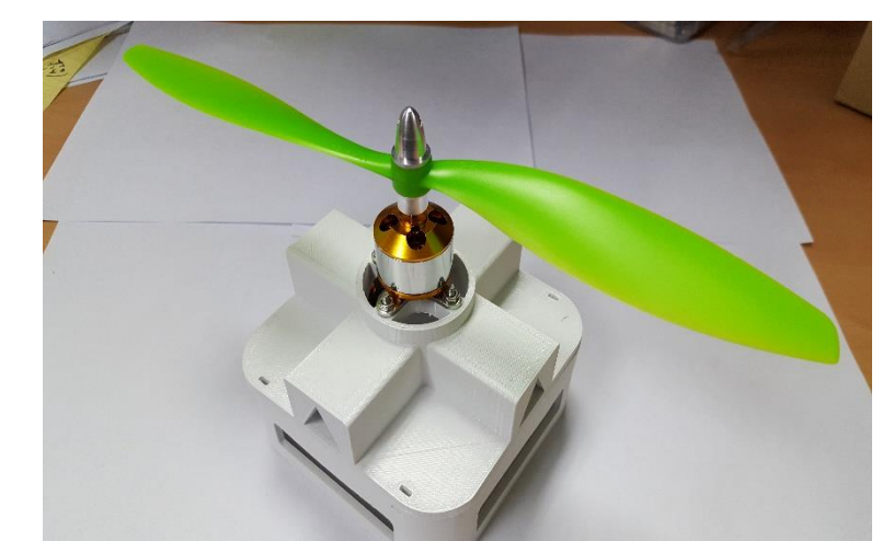
Figure 4. 3D Sketch of Final Prototype (Left: Upper Part for Motor and Rotor, Right: Bottom Part for STM Board and ESC)
